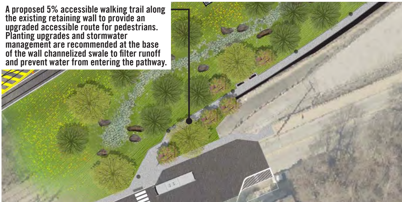
Conceptual design showing an ADA-compliant path, greenspace, and gateway upgrades to welcome all users to South Hills Junction.
