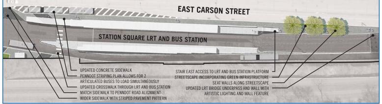
[Station Design] Conceptual master plan for Station Square LRT and Bus Station
